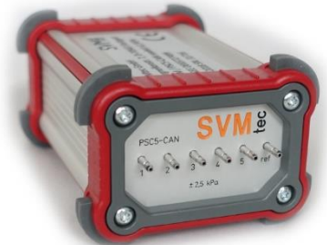
Figure 2: PSC5 in IP65 housing (custom version)
